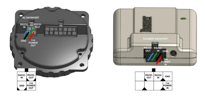
In the majority of instances, the Roamer should be powered by POWER OUTPUT of the A2 Autolube. However, if an alternate power source is required the Roamer works on 9VDC – 33VDC.
