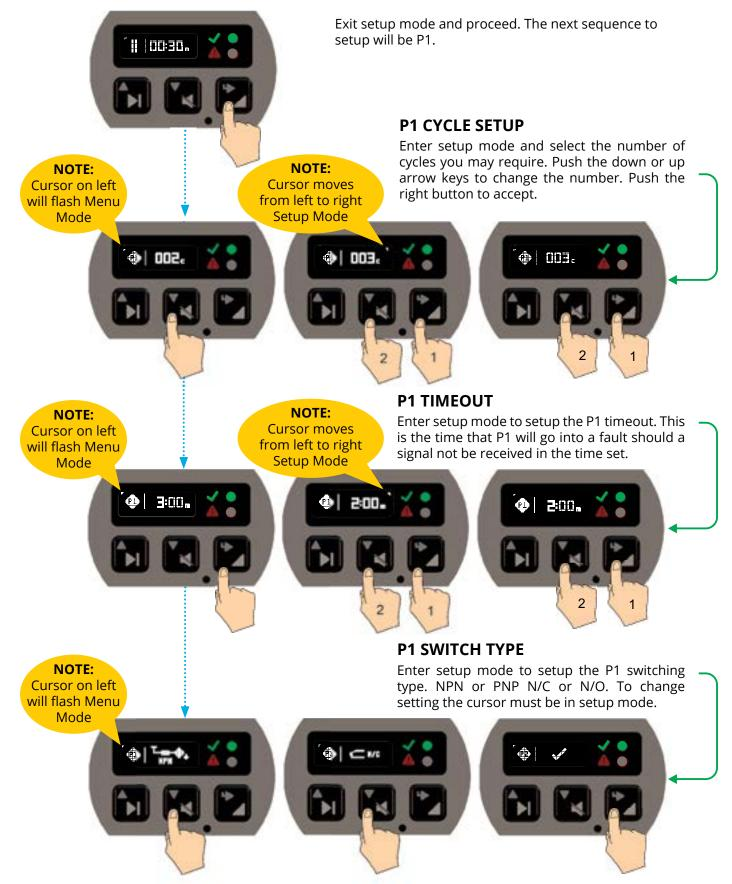
**NOTE:** For SLS using 2 pressure switches user must accept P2 as part of setup. Should P2 indicate X then enter setup mode and change to accept P2.
