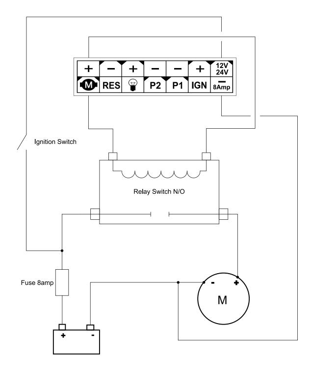
**NOTE:** Connect through vehicle fuse box to 15Amp fuse for standard equipment. High current equipment to rate fuse and wire up accordingly
