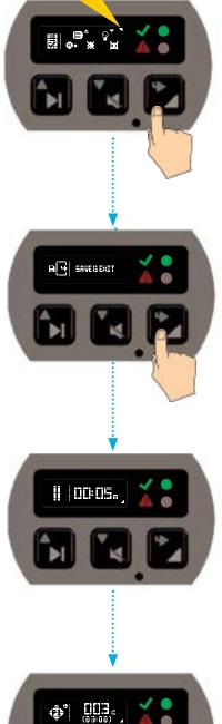
Display indicates selection accepted. Icons with X through are not selected. Push the right button to enter the TEST screen function. While is test mode user can press the middle button to test external warning light for function. Push the left button will switch the pump on. Should you have sensors connected such as proximity or low level the display will show if these are working correctly if activated. By testing the pump function will test proximity or pressure sensors.
