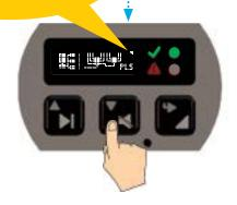
The screen now displays the type of lubrication system to setup. Press the centre button to select either PLS or SLS Note the flashing cursor on the right. This is an indication that you have entered the setup mode.
