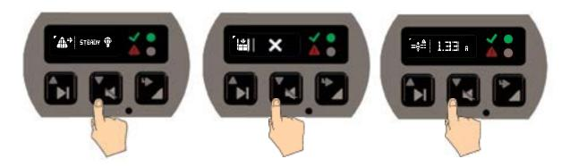
Continue to press the middle button to the next display. The next display will indicate external lamp warning. Setup for a steady output or flashing output. Continue to press middle button with option to setup low level. The next display will show blockage detection. Enter setup mode to set current draw for pump to stall.
