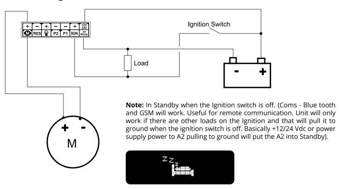
**Note:** Connect through vehicle fuse box to 15Amp fuse for standard equipment. High current equipment to rate fuse and wire up accordingly.
