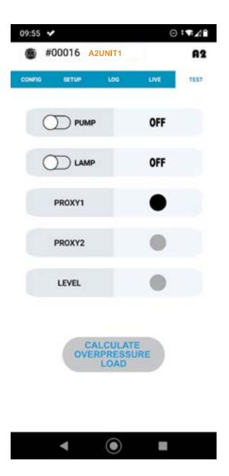
Used to test the system. When the app enters Test Mode, the A2 will also enter Test Mode and show this on its screen. The pump can be turned on and off, and when running will show the pump current draw (which can be used to calculate overpressure limits). The lamp can also be turned on and off. Proxy's and other settings are also shown.
