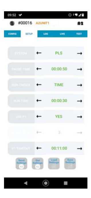
All settings on the A2 can be viewed and changed via the app. When the A2 is first connected the current settings from the A2 will be shown in green. When you make any changes to the settings the text will update to red, however these will only be applied to the A2 when they are specifically sent. This enables users to finalise the required settings before sending them to the A2.
