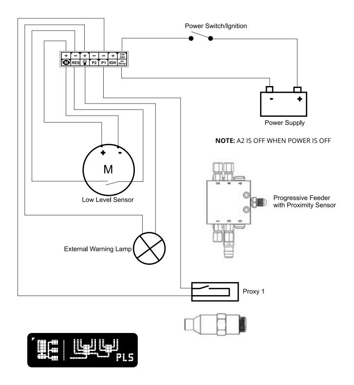
**NOTE:** Connect through vehicle fuse box to 15Amp fuse for standard equipment. High current equipment to rate fuse and wire up accordingly.
