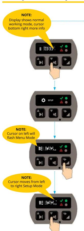
**NOTE:** The cursor to the right bottom of display indicates more information available. Press the right button key to access the stored information. Information stored shows Hours worked, total hours paused and all accessories connected hours performed.
