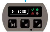
Run timer will display after the default pause time expires. The left "Play" arrow will flash together with the green LED. This indicates that the pump is running.
