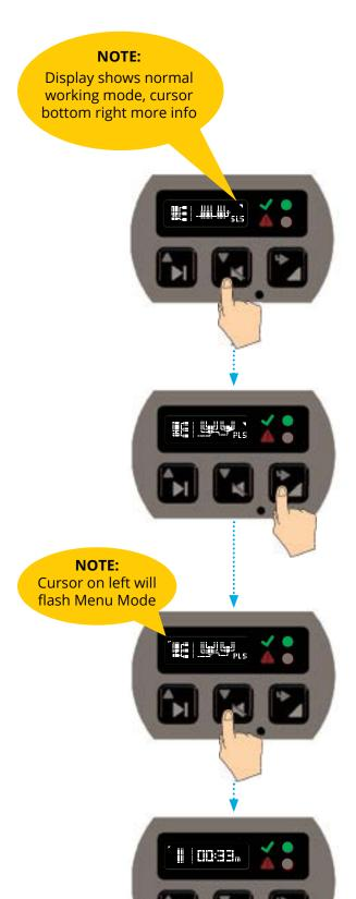
Press the centre button to select from SLS to PLS. Note the flashing cursor on the right. This is an indication that you are still in setup mode.
