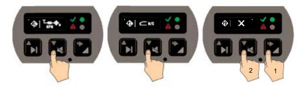
Enter the setup mode to set P1 switching type. NPN or PNP normally closed or open are options to consider and depending on the sensor type installed. To change setting the cursor must be changed from menu mode to setup mode. Enter X (No) for P2.
