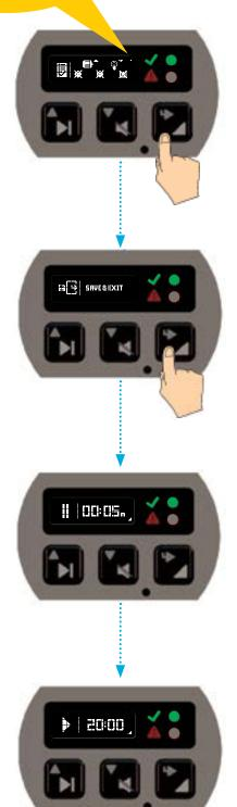
Display indicates selection accepted. Icons with X through are not selected. Push the right button to enter the TEST screen function. While is test mode user can press the middle button to test external warning light for function. Push the left button will switch the pump on. Should you have sensors connected such as proximity or low level the display will show if these are working correctly if activated. By testing the pump function will test proximity or pressure sensors.
