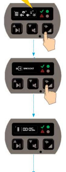
Display indicates selection accepted. Icons with X through are not selected. Push the right button to enter the TEST screen function. While is test mode user can press the middle button to test external warning light for function. Push the left button will switch the pump on. Should you have sensors connected such as proximity or low level the display will show if these are working correctly if activated. By testing the pump function will test proximity or pressure sensors.
