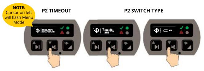
**NOTE:** P2 timeout and normally represents the low pressure sensor will by default close first. The timeout for P2 can be set at the same time as P2. Should a signal not be received within 2 mins for P1 or P2 the system will go into a fault. P2 Switch type should be setup as P1 or in the case where P2 sensor type is different. User will need to have knowledge of the type of sensor used.
